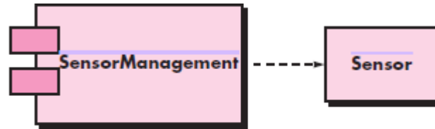
Fig 8.6: A UML component diagram
