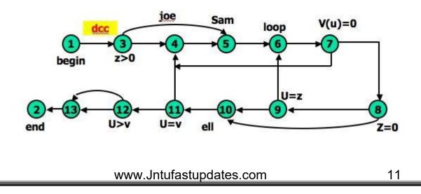
Figure 3.9: Control flowgraph annotated for X and Y data flows.
